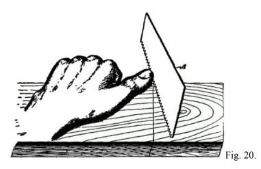
The Starting Cut.—In order to make our understanding of the starting cut more explicit, we refer to Fig. 20, in which the thumb of the left hand is shown in the position of a guide—the end of the thumb being held up a sufficient distance to clear the teeth. In this position you need not fear that the teeth of the saw (A) will ride up over the thumb if you have a firm grasp of the saw handle.
